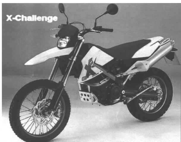
On the X-Challenge Hard Enduro design, the front fork offers 25 cm of travel and is tuned specifically to off-road use, with the unit adjustable for compression and rebound damping. The rear suspension is the most different from the other two 650s, as it employs the Air Damping System showcased on the HP2. The rear suspender works like a conventional spring unit but utilises pressurised air, with the rider able to use a high-pressure pump located underneath the seat to adjust the unit.
